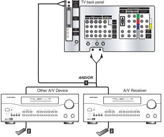
**Figure 2.** Connecting the IR Home Theater Control and/or Repeater.
